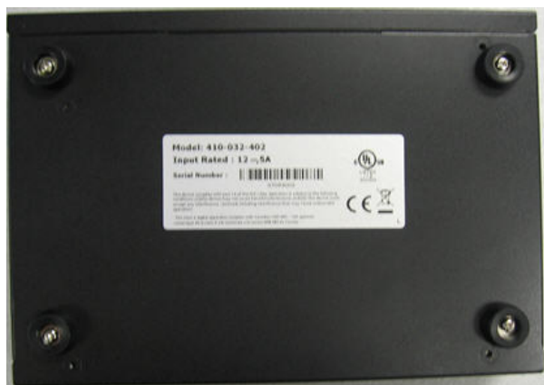
Figure 20 Rubber feet installed
